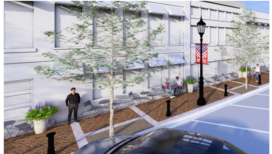
Typical sidewalk section incorporates 5'-0" min clear walking space flanked by 2-tops adjacent to building facades and decorative lighting, bollards and tree plantings along the roadway curb.
