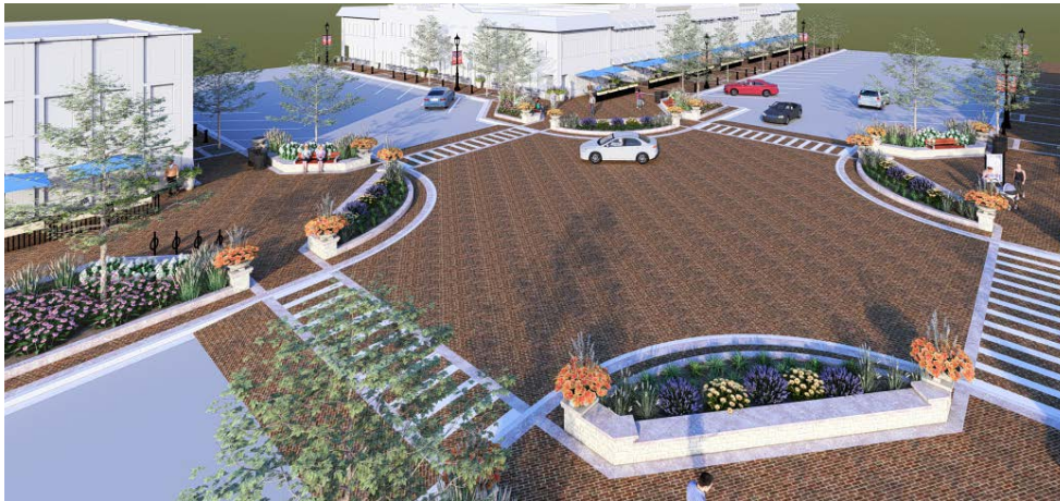
Raised intersection area calms traffic and prioritizes pedestrian crossings. Bumpouts are enhanced with stone seatwall planters, bike racks, decorative planter pots and decorative unit pavers. Where sidewalk widths allow, sidewalk cafes are defined by perimeter cafe railings and planters.
